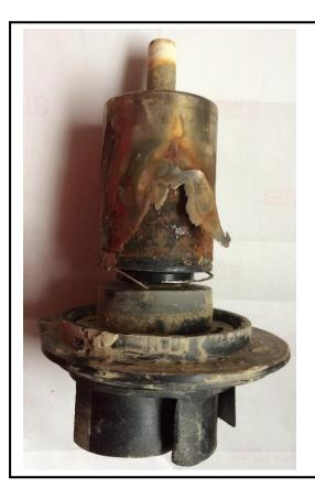
If your rotor looks similar to this one, please check inside the main housing to ensure it is not damaged. Typically, we can start by trying a new rotor to get your pump back up and running, as long as, the main housing is not damaged.
