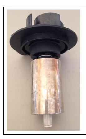
This picture is what your rotor should look like after it is cleaned. Please make sure that the ceramic shaft and silver plating are both still intact after disassembling and cleaning.
